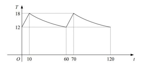
The temperature is controlled by a thermostat such that when the temperature falls to  $12^{\circ}$ C, a heater is turned on until the temperature reaches  $18^{\circ}$ C. The room then cools until the temperature again falls to  $12^{\circ}$ C.
